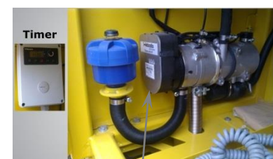
HEATING SYSTEM FOR ENGINE
