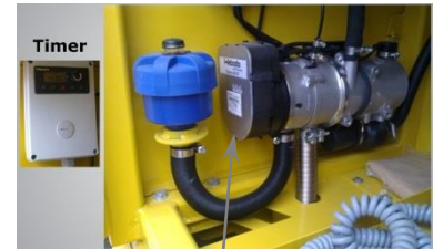
HEATING SYSTEM FOR ENGINE
